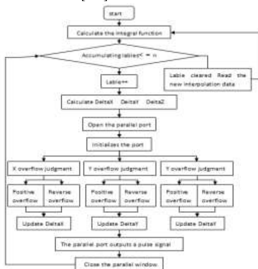
Fig.1 Flow chart of position control module
